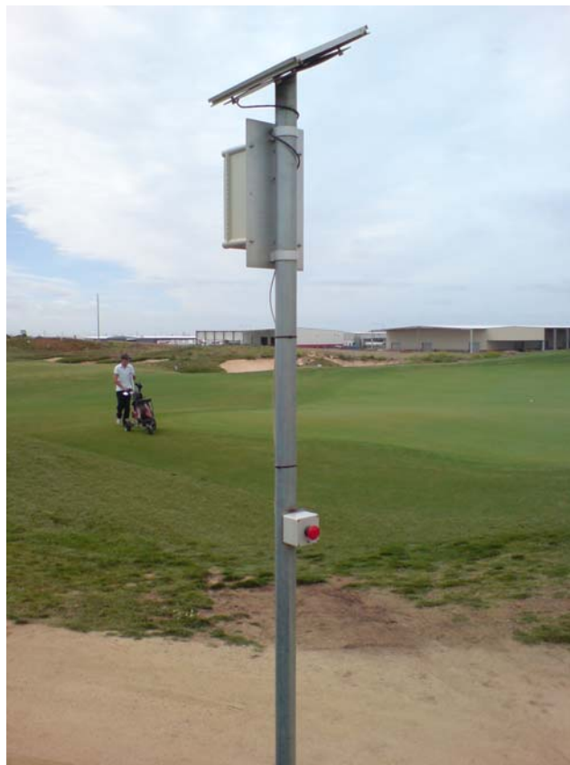
TeeSafe™ showing the solar panel, lights and button for activating and deactivating lights.
